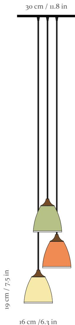
\* Please supply required drop length, measured from the ceiling to the bottom of the fitting at the time of order.
